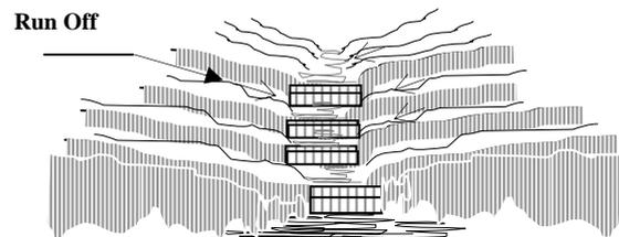
Gambar 2.10 Gully Stabiliation ( Gully Plug).
